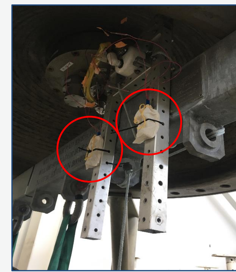
Cases were placed inside bags in case they shattered or failed
