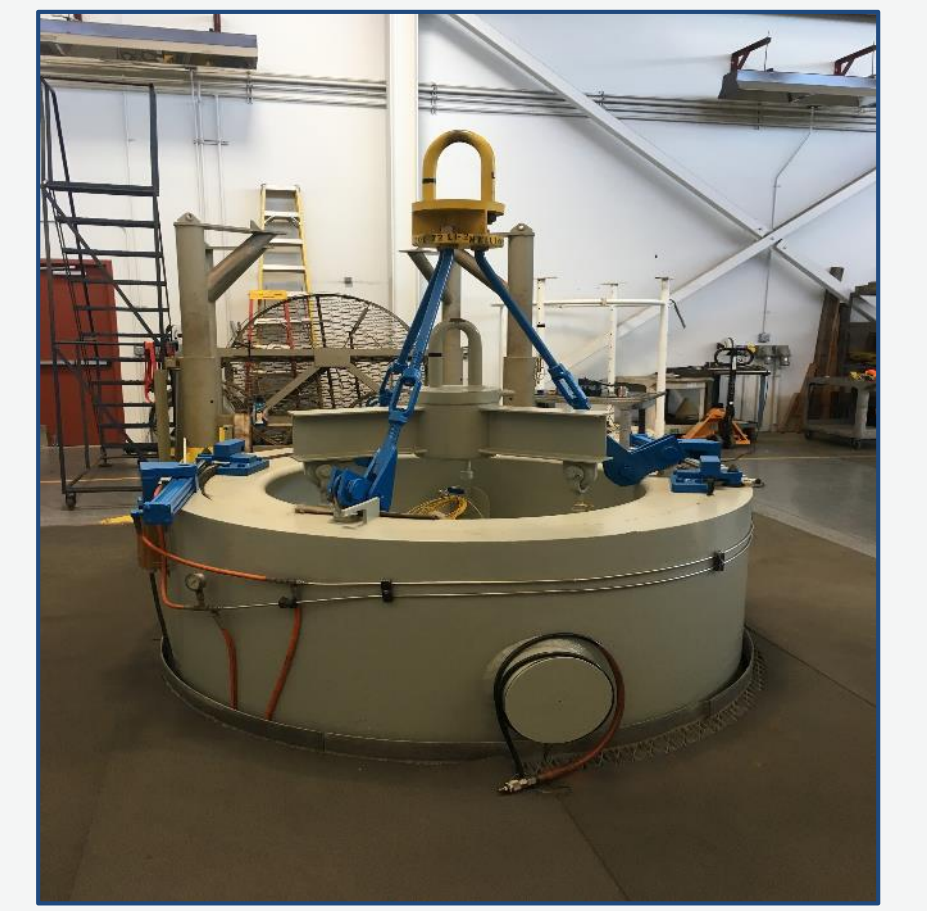
Pressure vessel sealed with the prototypes inside
