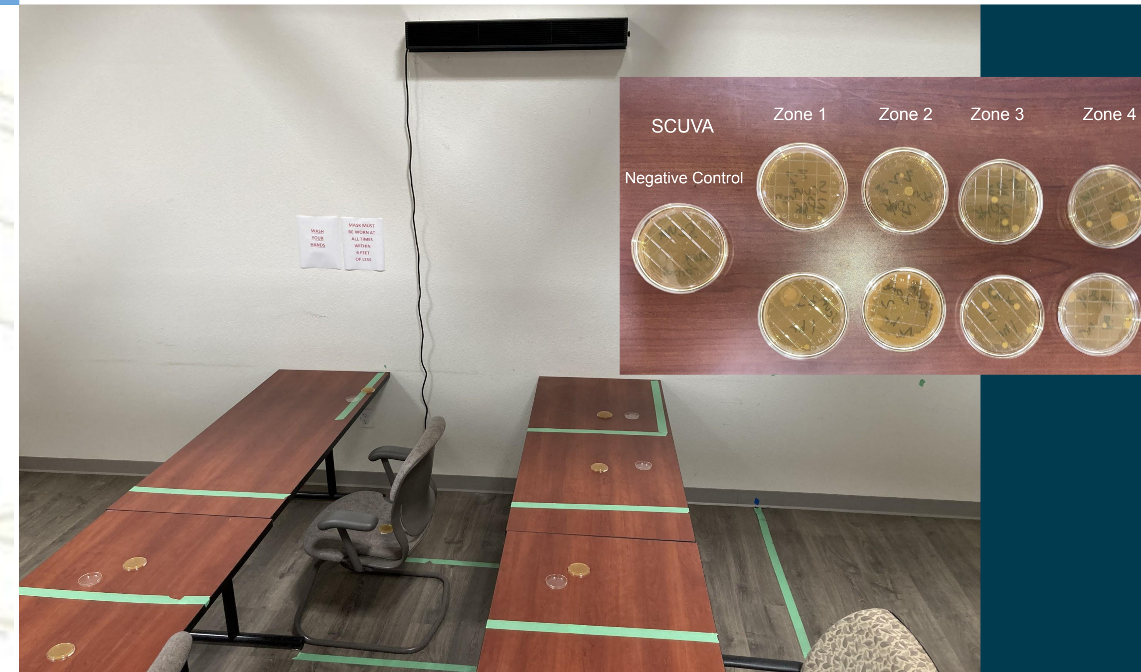
Left: Testing set up for UV Light Solutions system. Right: Incubated samples from SCUVA T400 testing.
